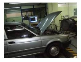
Vehicle on rollers dynamometer
